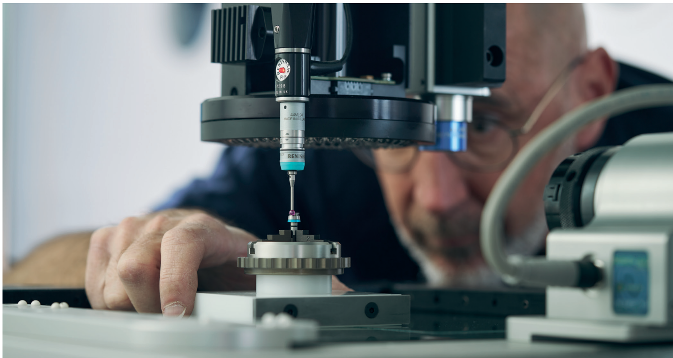
Part measurement by probing on a MicroVu VERTEX 312 machine
