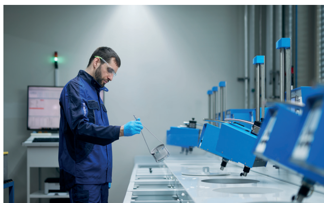
Manual leaching and/or passivation
