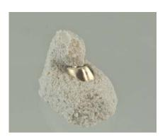
The solder gap should be continuous and between 0.05-0.20 mm wide. Then design the soldering block, so that the male part is securely held and good flame access is ensured (observe corresponding solidus).
