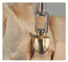
Then place the CM LOC® male part E and laser weld around circumference.
