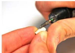
Roughen the surface using a diamond milling cutter and clean with alcohol before sandblasting the framework.
