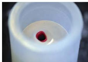
Use a suitable instrument for the fine investment of the cavity (e.g. small brush), so that the humidity will not be withdrawn from the investment material.
