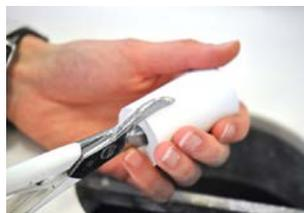
Fine divestment is carried out with abrasive 110µm aluminum oxide under pressure of 2 bars.
