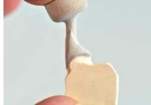
Cut the sprue by using a cutting wheel.
