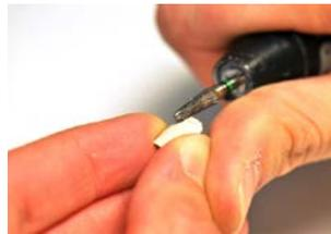
Roughen the surface using a diamond milling cutter before sandblasting the framework.
