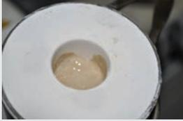
PEKKtherm remains closed for 20 minutes followed by an alarm (beep). Press the Go button, furnace opens.
