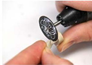
Cross-toothed milling is used to finish the framework.
