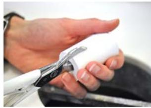
Fine divestment is carried out with abrasive 110 $\mu$ m aluminum oxide under pressure of 2 bars.
