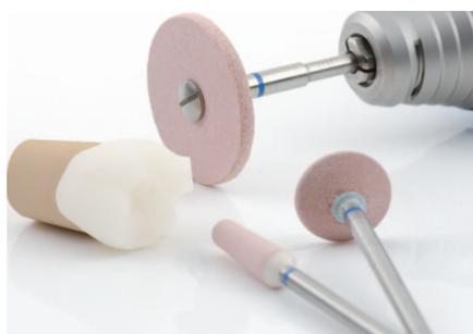
Separation from cone with diamond cutting disk.
