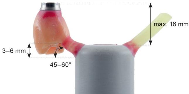
Tip: When sprueing one hybrid abutment crown only, fit a pressure compensation channel!
