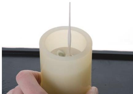
Set shaker to minimum stage. Fill material carefully but swiftly to the rim of the object. Then fill the object carefully bubble-free until it is covered completely.
