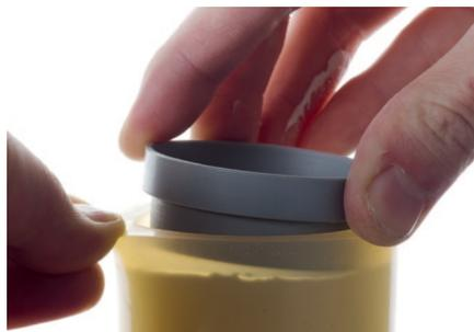
Once the object is covered, switch off the shaker and fill the investment ring up to the marking with the remaining investment material. Slightly push out the silicone rim of the investment ring and place the ring lid and rotate once clockwise by 180° (elimination of bubbles).
