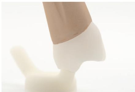
Result of a crown after cleaning, without any finishing, with attached stump.
