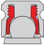
The retention force is adjusted by turning clockwise to increase the retention force and vice versa to reduce the retention force. The maximum retention force is approx. 1200 g (lamellae retention insert cannot be screwed in any further).
