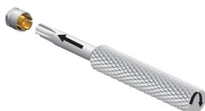
The screwdriver / activator (Cat.-No.072 609) is required to activate, deactivate and remove the lamellae retention insert. The instrument with four cams is pushed into the lamellae retention insert in its correct position up to the stop.
