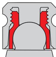
The basic setting on delivery is approximately 200 g, which also represents the minimum retention force to be set (lamellae retention insert is flush with the lower edge of the housing).
