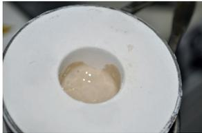
PEKKtherm remains closed for 20 minutes followed by an alarm. Press the Go button, furnace opens.
