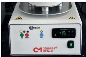
When the Go LED lights up green (audible beep), the device is ready for operation (at 390°C) and ready for programme selection.
