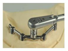
Torque for the CM LOC<sup>®</sup> CAD CAM Retention Element > 35 Ncm.
