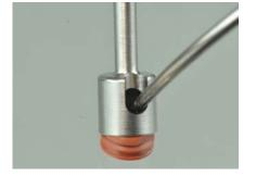
Then use an instrument to remove the CM LOC<sup>®</sup> Housing from the CM LOC<sup>®</sup> Housing Extractor through the side opening. For better removal, it is recommended to briefly warm the CM LOC<sup>®</sup> Housing Extractor over a flame.
