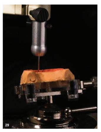
Mount the model on a surveyor table of a parallelometer unit and select the correct direction of insertion using the HexScan® Positioner 3mm. Fig.29. The so determined direction of insertion should then be valid for the rest of the teeth in the arch.
