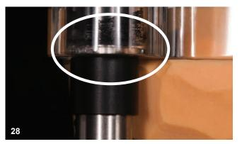
Always check that the verticulator is completely down in its home position before proceeding. Fig. 28
