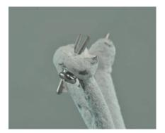
Fit the CM LOC<sup>®</sup> spacer to protect the male part while sandblasting and processing.
