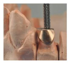
In a first step, face mill the root canal cap using a milling machine at right angles parallel to the direction of insertion.
