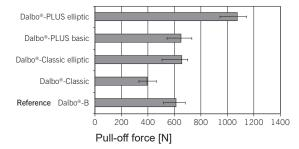
Comparison of retention force of Dalbo® Female parts in the denture body All ball female parts demonstrate sufficient retention in the denture body under laboratory conditions. Remarkable is the high value of the Dalbo®-PLUS Female part elliptic, which in part even exceeds the mechanical properties of the resin.
