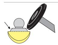
Refining the surface of the weld. In order to guarantee the stability of the laser-welded joint, avoid grinding off too much material.
