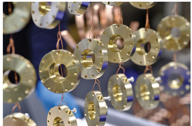
Parts prepared for the surface treatment process at R. Schlierholz
